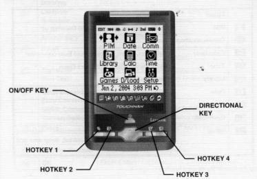
There are also five keys below the LCD screen: four 'hot keys' and a larger Up / Down key in the middle. Hot keys start applications and they are fixed. Their default settings are as follows (from left to right):
